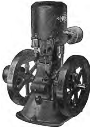
FIG. 181.—Electrical Gas Engine. Notice the two fly-wheels and the pulley attached on the left. Power is transmitted from the pulley by means of belting.
